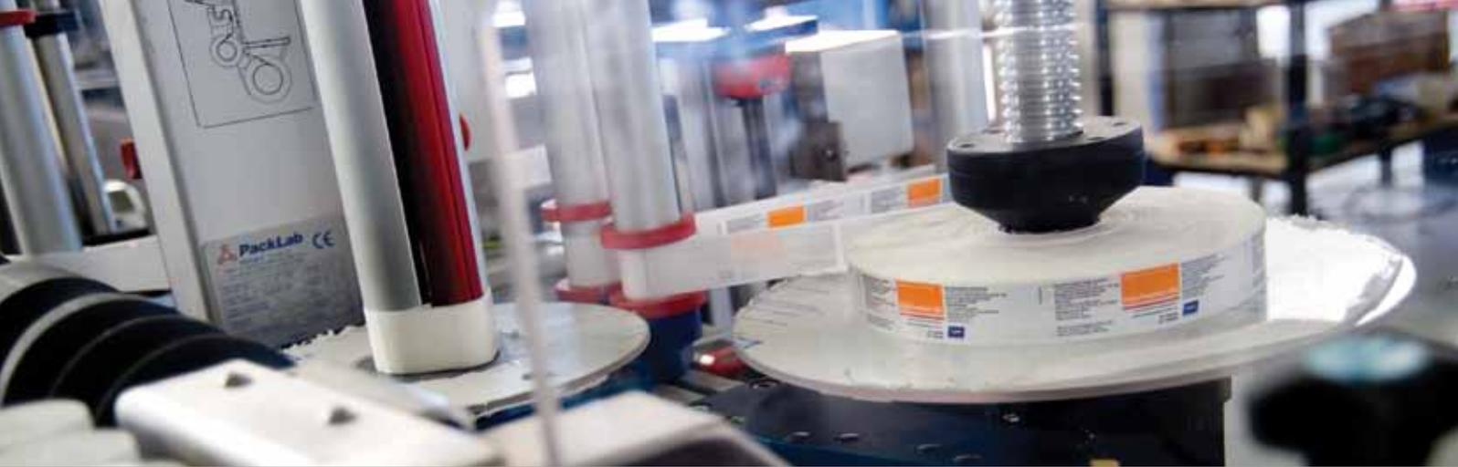
**Labellers** are specifically designed and customisable to customer requirements and are available in a number of configurations including single, or twin labelling heads with PLC control and interlocked glass/polycarbonate guarding as optional extras.
